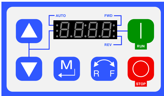
Figure 15 Painel de Controlo do VFD
