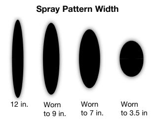
Example: When a tip that had a 12-inch fan pattern is reduced to a 9-inch fan when worn, it will output 40% more paint on 25% less area. Overlapping to achieve a consistent mil thickness becomes impossible. The chart above illustrates the effects of a worn tip on a spray pattern.
