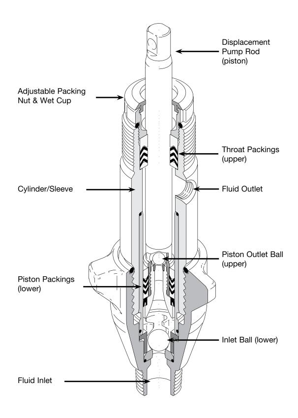
The general purpose of the packings is to create a seal and direct fluid flow. There are two sets of packings, *throat* and *piston*:
