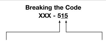
First 1-2 digits when doubled, is spray pattern fan width. A 515 has a 10-inch fan width when sprayed 12 inches from surface.
