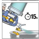
Note: Store Sprayer filled with Pump Armor" (included) storage fluid for trouble-free startup.
