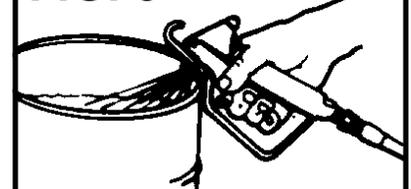
MAINTAIN FIRM METAL TO METAL CONTACT BETWEEN GUN AND CONTAINER
