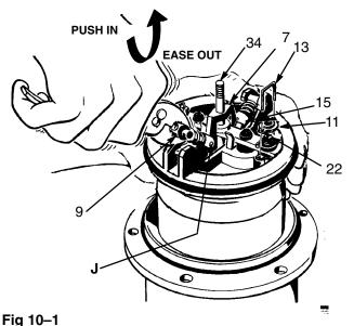
Grip the toggle rockers (9) with a pliers. Compress the springs up, away from the piston lugs, and remove the parts. Check to see that the valve actuator (33) is supported by the spring clips (38), but slides
