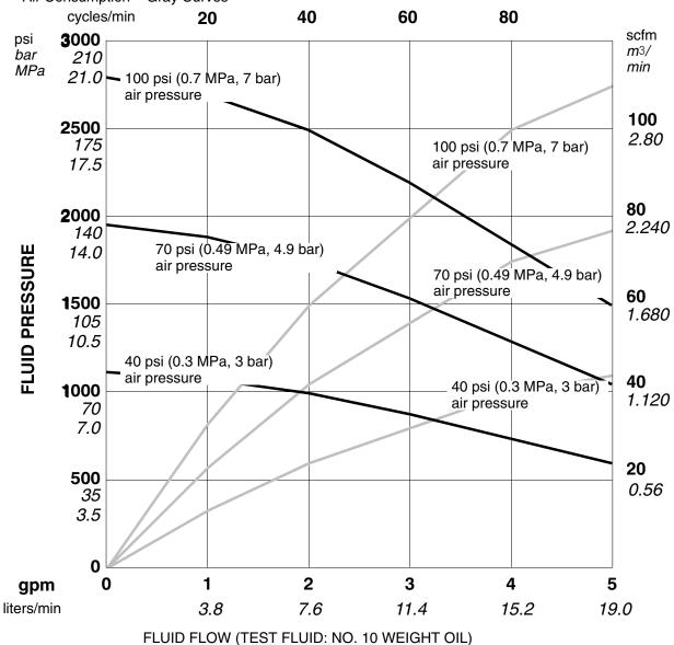
**To find Fluid Outlet Pressure** (bar/psi/MPa) at a specific fluid flow (lpm/gpm) and operating air pressure (bar/psi/MPa):
