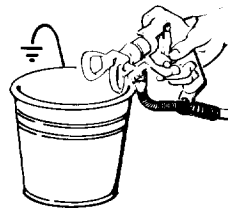
DISENGAGE SAFETY AND TRIGGER GUN; ENGAGE SAFETY AGAIN
