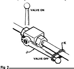
5. When this gun is pressurized, opening the ON/OFF lever releases high pressure fluid suddenly which causes the front end of the pole gun to pull up or "kickback". To reduce the effect of the kickback, *always* grasp the grip (L) firmly with one hand, be sure you have a good footing, and open the ON/OFF lever with your other hand, See the Typical Installation drawing, page 4.
