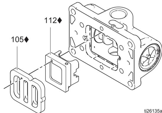
Air Valve Disassembly or Reassembly
