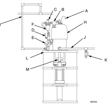
4. Install the air line accessories in the approximate order shown. To reduce stress on the air inlet fitting, do not mount any accessories directly at the air inlet fitting. Mount accessories on a bracket or other fixture and use a hose between the accessories and air inlet. Use the shortest practical length of hose.
