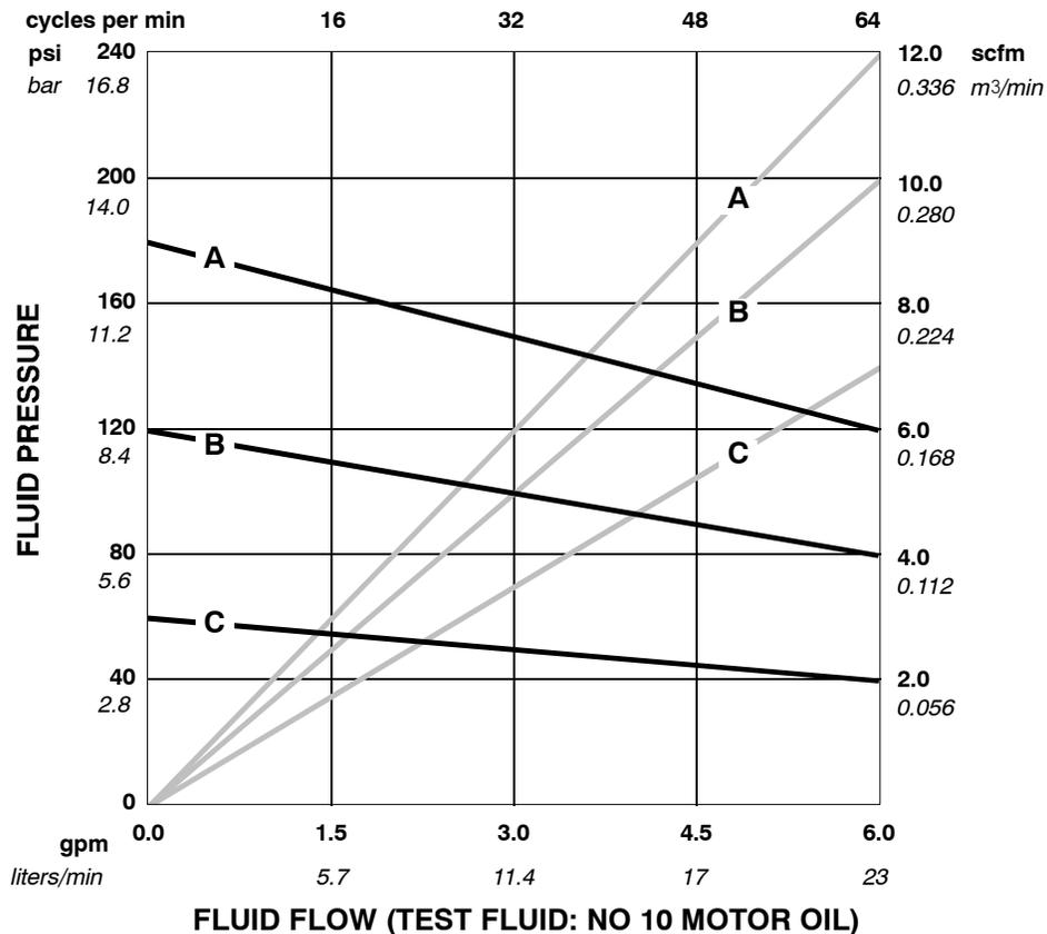
**To find Fluid Outlet Pressure** (bar/psi) at a specific fluid flow (lpm/gpm) and operating air pressure (bar/psi):
