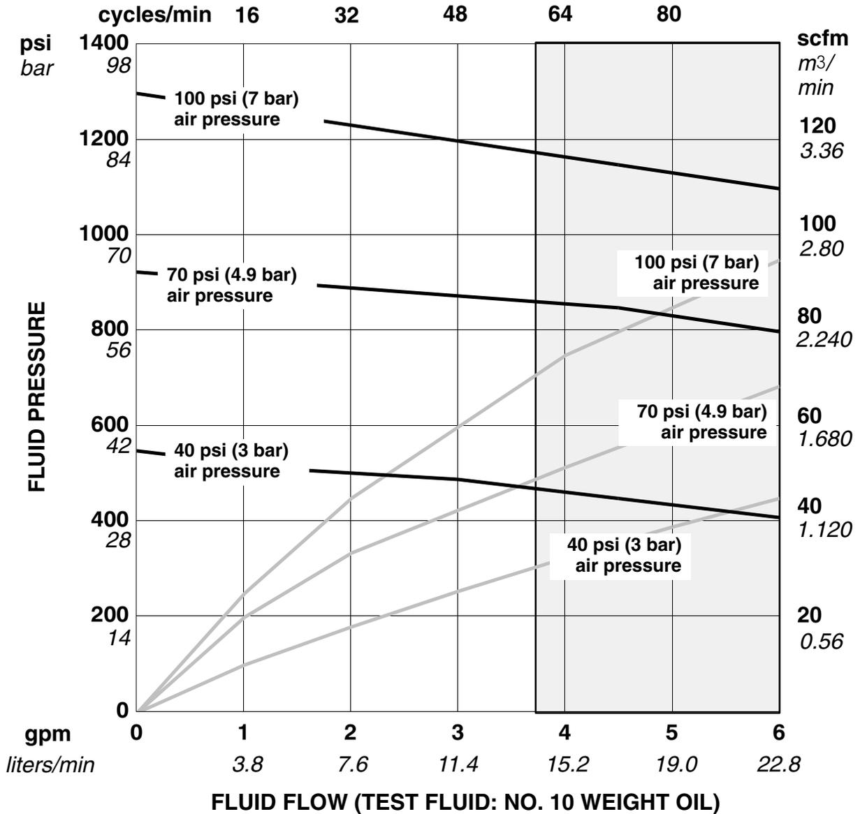
**To find Fluid Outlet Pressure (bar/psi) at a specific fluid flow (lpm/gpm) and operating air pressure (bar/psi):**
