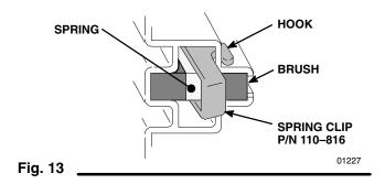
4. Loosen the brush lead terminal screw. Pull the brush lead away, leaving the motor lead terminal in place. Remove the brush and spring. See Fig. 15.
