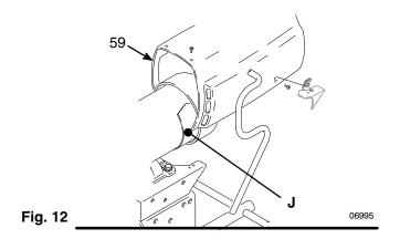
Push in the spring clip to release its hooks from the brush holder. Pull out the spring clip. See Fig. 13.
