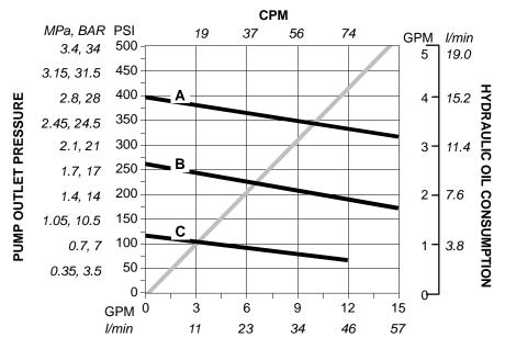
PUMP DELIVERY (Test Fluid: No. 10 Motor Oil)
