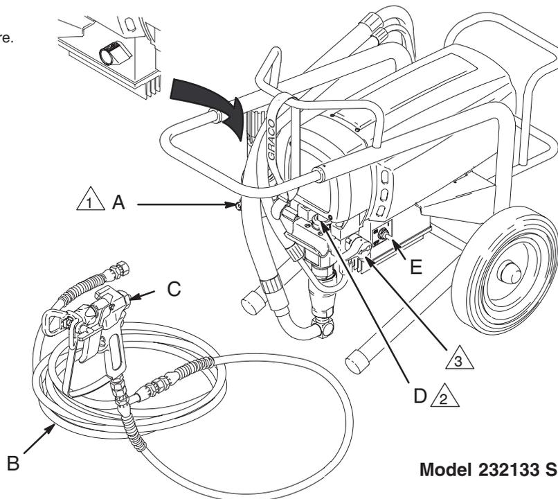
2. **Fill packing nut (D).** Fill packing nut full with Graco Throat Seal Liquid (TSL) (64) supplied.
