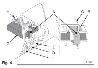
Inspect commutator for excessive pitting, burning or gouging. A black color on commutator is normal. Have commutator resurfaced by a qualified motor repair shop if brushes wear too fast.
