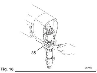
Fig. 19. Screw jam nut down onto pump until stops. Screw pump up into bearing housing until it is stopped by jam nut. Back off pump and jam nut to align pump outlet to back. Tighten jam nut by hand, then tap 1/8 to 1/4 turn with a 20 oz (maximum) hammer to approximately 75  $\pm$  5 ft-lb (102 N·m).
