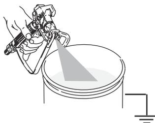
4. Engage trigger lock. See Trigger Lock, page 10 or your gun operation manual.
