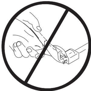
Only use an **extension cord** with an undamaged 3-prong plug. Recommended extension cords for use with this sprayer:
