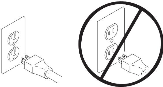
Do not use the sprayer if the electrical cord has a damaged ground prong.
