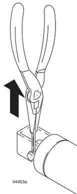
4. Gently push cylinder forward, relieving tension on pin. Pull out pin.
