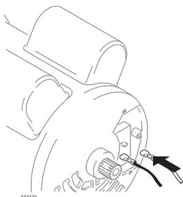
8. Reattach green ground wire and grounding nut.
