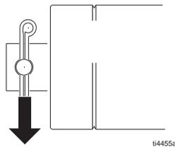
6. Replace cotter pin through hole in pin, bending ends to secure.
