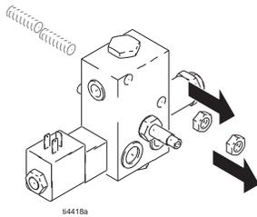
5. Remove Relief Valve from sprayer frame.
