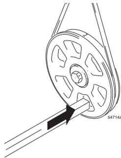
2. Remove large bolt and washer in center of rotor assembly.
