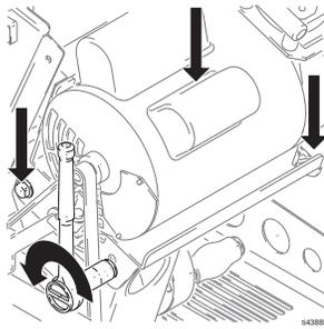
2. Loosen 2 bolts (1 each side) holding down support rod.
