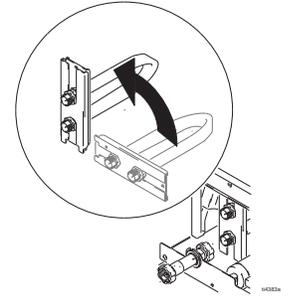
6. Slide pump hose around rollers. Make sure the rollers are horizontally parallel to each other.
