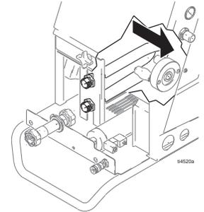
7. Slide feet on the bottom of hose bracket, into the slot on the bottom of sprayer.
