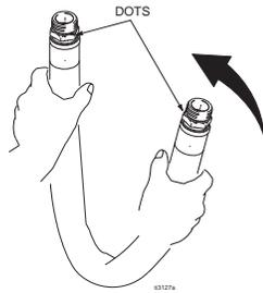
2. Insert hose ends through holes in inner hose bracket, keeping dots on fittings facing each other and kinked portion of hose horizontal to the underside of bracket.
