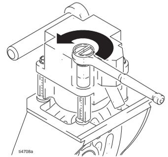
6. Remove bolts and housing from motor.
