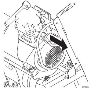
7. Remove 3 screws on right side of cover and remove cover.
