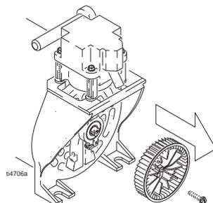
4. Remove 3/8 in. bolt holding piston to motor shaft.
