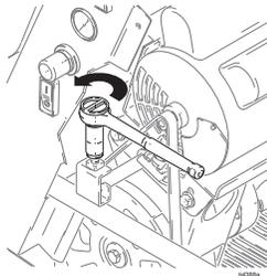
3. Using a screw driver for leverage, lift up on motor support rod on one side of motor and ease it out of the holding bracket far enough to remove old belt. Discard old belt.
