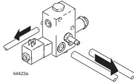
4. Remove 2 nuts securing Relief Valve to sprayer.
