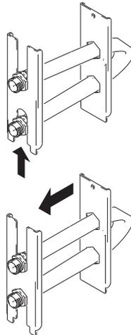
4. Slide plates together, inserting inner plate in outer plate, matching alignment holes.
