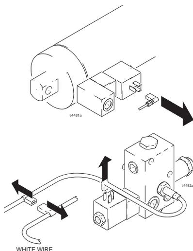
2. Rotate counter-clockwise to remove sensor from manifold.
