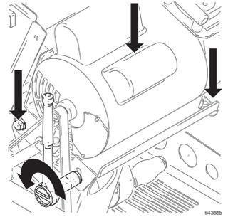
5. Slide belt off motor pulley.
