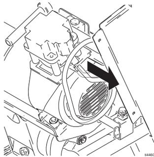
2. Remove 3 screws in side of motor cover. Remove cover.
