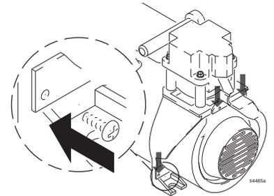
8. Reconnect air line from motor to cooler.
