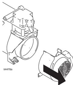
3. Remove fan bolt from center of fan and remove fan from housing.
