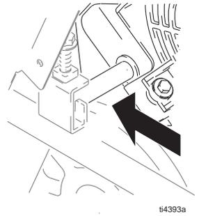
3. Insert crow bar under assembly as shown and raise motor assembly until desired belt tension is achieved.
