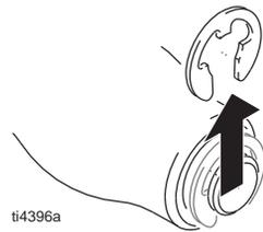
2. Remove roller assembly from rotor pins (a).
