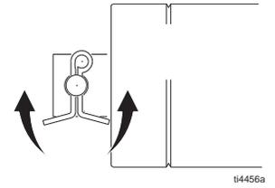
7. Reattach electric wire terminals. Terminals are not polarity sensitive and can be connected to either post.
