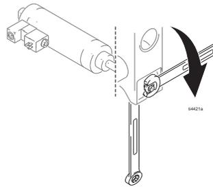
3. Install locking nut flush to end of shaft.
