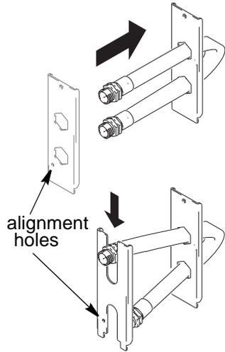
3. Slide hose ends into outer hose bracket, making sure dots on fittings face each other and alignment holes are together (slide into long slot first).
