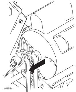
6. Disconnect air line from compressor to cooler and remove.
