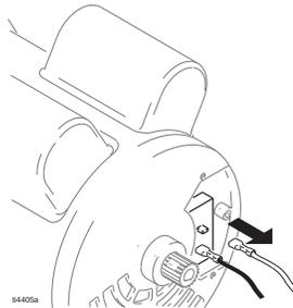
4. Loosen 4 bolts (2 each side) to loosen tension on belt.
