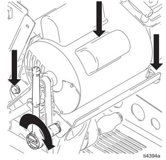
6. Turn belt one more time with your hand to make sure teeth are properly engaged and tension is correct.
