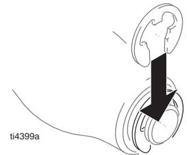
4. Replace back and front covers and hopper. See Removing and Replacing Hopper, Front and Back Cover, page 9.
