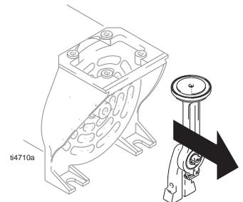
8. Using parts in kit replace piston, seals and sleeve.
