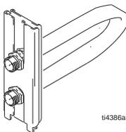
5. Replace bracket assembly in housing making sure the mounting screw hole, located in the top center of the inner plate, faces up.
