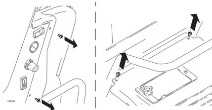
2. Lift cover up and then tilt it back and off sprayer frame.
