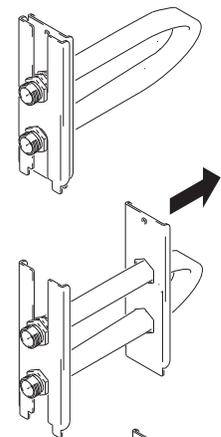
6. Slide hose ends out of slots in outer hose bracket (slide out of short slot first).
