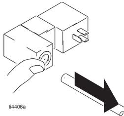
2. Remove electric wire terminal connections.
