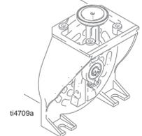
7. Remove piston rod from motor.
