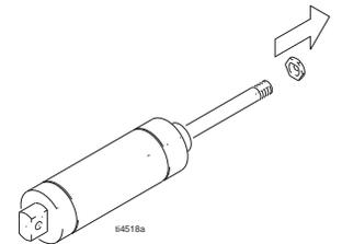
7. Using a 15/16 in. wrench, loosen nut, located inside sprayer frame at the end of the air cylinder.
