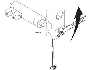
8. Using a 15/16 in. wrench, loosen nut on the other side of the sprayer frame.
