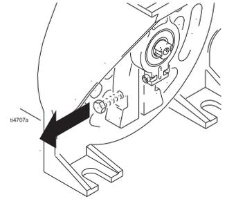
5. Loosen 4 bolts on top of motor housing.
