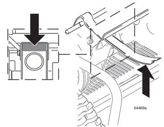
4. While holding motor assembly in place with crow bar. Spin pulley to assure proper belt engagement. Adjust motor assembly position as necessary.
