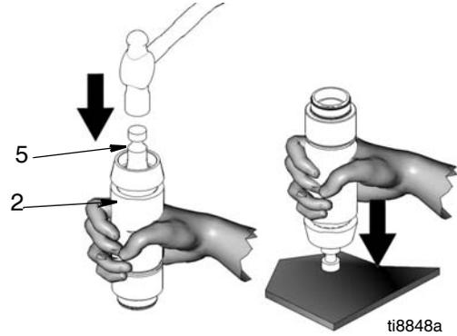
5. Remove piston rod (5) from sleeve (4).
