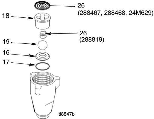
15. Install intake valve on cylinder. Torque to: 200 +/- 15 ft-lb (271 +/- 20 N•m) for 288467, 288468, 288819, 24M629; 110 +/- 5 ft-lb (149 +/- 7 N•m) for 24B748.
