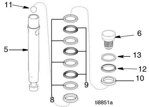
8. Remove throat packings and glands from cylinder. Discard throat packings and glands.
