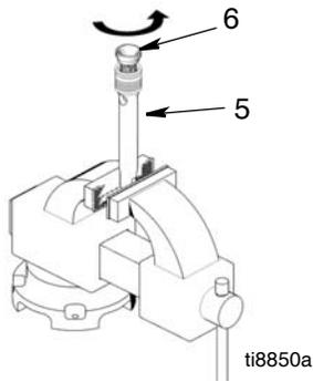
7. Remove packing and glands from piston rod. Note orientation for installation.
