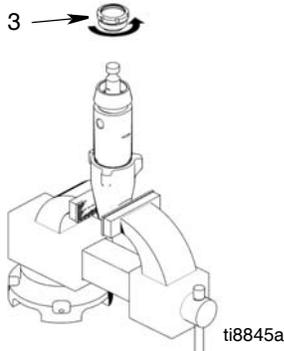
2. Unscrew intake valve from cylinder.
