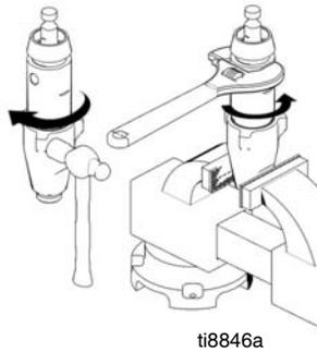
3. Disassemble intake valve. Clean and inspect o-ring (17). You may need to use a pick to remove o-ring. **NOTE:** Spring (26) for model 288819 is optional and is not included with the pump.
