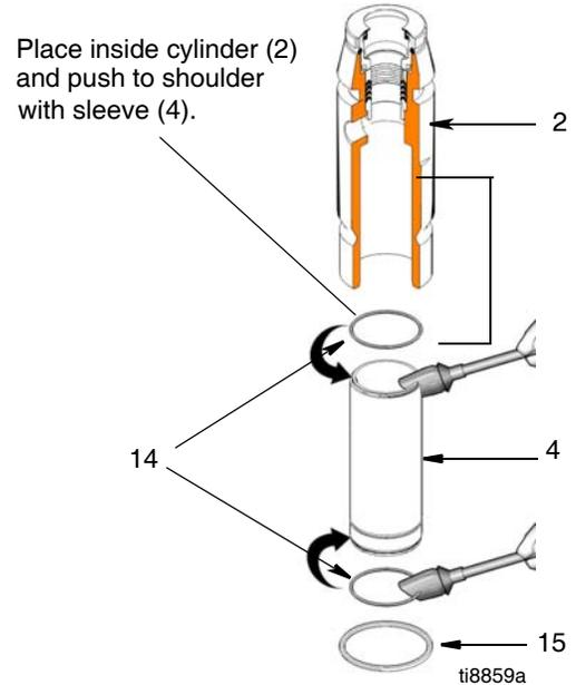
**NOTE:** O-ring (15) is not required for safe pump operation.
