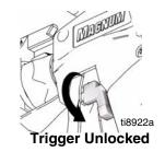
Hold gun firmly to side of pail. Trigger the gun to relieve pressure.
