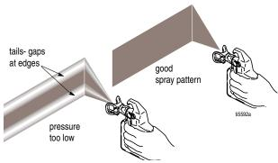
If tails persist when spraying at the highest pressure, a smaller tip is needed or the material may need to be thinned.
