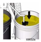
7. Submerge suction tube in water or flushing solvent.
