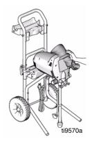
To avoid overheating motor, keep vent holes in shroud clear for air flow.
