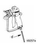
12. Wipe paint off outside of gun using a soft cloth moistened with water or flushing solvent.
