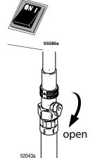
Open lever on Power Flush attachment.
