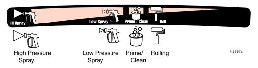
To select function, align symbol on pressure control knob with setting indicator on sprayer.
