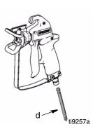
Clean tip and guard with water or flushing solvent. A soft brush can be used to loosen and remove dried on material if needed.
