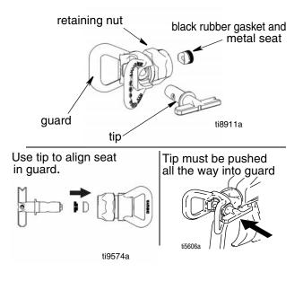
3. Screw tip and guard assembly on gun. Tighten retaining nut.
