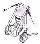
The folded sprayer can be stored on a wall as shown.
