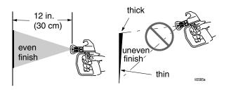
Flex wrist to keep gun pointed straight. Fanning gun to direct spray at angle causes uneven finish.
