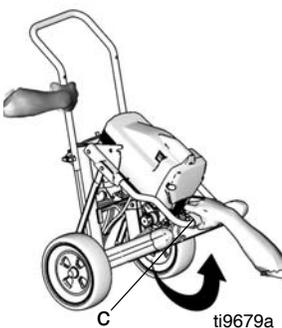
4. Install hose rack (d) to frame handle. Install lock nuts. Tighten securely.
