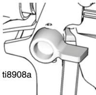
Trigger Locked SG20, SG2, SG3, SGPro
