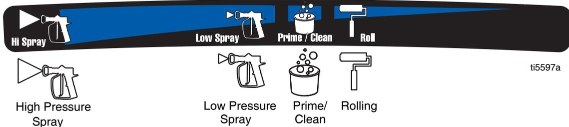
**NOTE:** To select function, align symbol on pressure control knob with setting indicator on sprayer.
