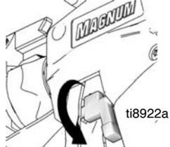
Trigger Unlocked SG10
