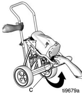
4. Install hose rack (d) to frame handle. Install lock nuts. Tighten securely.
