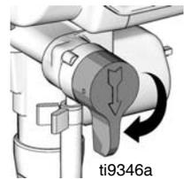
3. Hold gun firmly to side of pail. Trigger the gun to relieve pressure.
