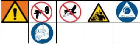
This equipment stays pressurized until pressure is manually relieved. To help prevent serious injury from pressurized fluid, such as skin injection, splashed fluid and moving parts, follow the **Pressure Relief Procedure** whenever sprayer is stopped and before sprayer is cleaned or checked, and before equipment is serviced.
