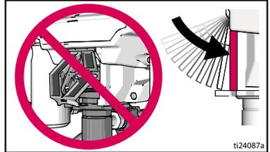
5. Use both hands to tighten pump retaining nut.
