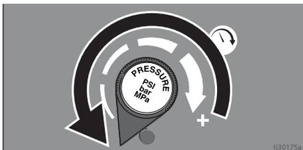
4. Put drain tube into a waste pail and turn Prime/Spray valve in PRIME position (drain) to relieve pressure.
