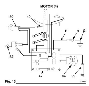
When turning the fan on a DC motor, normally you sense an even, pulsing resistance. If there is irregular turning resistance, or no turning resistance, check and repair the following as needed: broken brush springs, brush leads, motor leads; loose brush terminal screws or motor lead terminals; worn brushes. See page 21.
