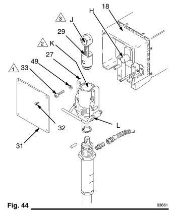
**NOTE:** Stop the sprayer at the bottom of its stroke to get the crank (H) in its lowest position. To lower the crank manually, rotate the blades of the motor fan with a screwdriver.
