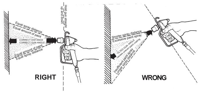
Hold the spray gun 12 - 15 inches away from the work surface and keep it perpendicular (straight) to the surface. Move the spray gun parallel to the work and at a right angle to the surface.
