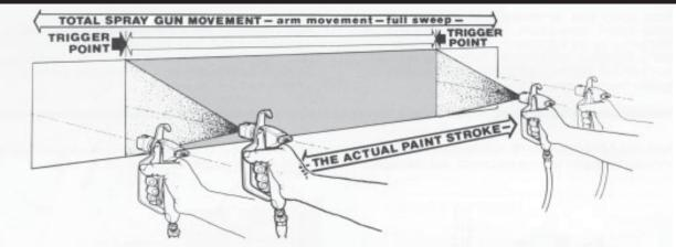
It is important to "trigger" the gun after gun movement (arm movement) has started and release trigger (shut gun off) before gun movement ends. Gun movement is always longer than actual paint (spray) stroke. In that manner, even blending and uniform paint coat thickness is achieved over the entire surface. When the gun is in motion as the trigger is pulled, it deposits an even amount of paint.
