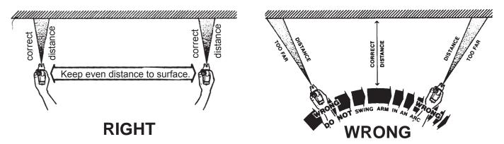
Move the gun at a steady rate in order to apply a good coverage. The wet coat should be just under the thickness at which a run or sag will occur Slow must be moved to prevent sags and runs. Holding gun movement or gun held too close will result in anthe gun too far from the work will cause excessive overly wet or thick wet or thick coat coverage that is likely to run or sag.
