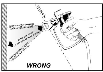
Hold the spray gun 12 - 15 inches away from the work surface and keep it perpendicular (straight) to the surface. Move the spray gun parallel to the work and at a right angle to the surface.
