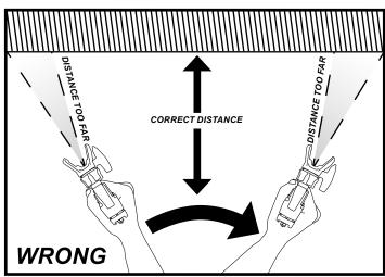
The closer the spray gun is held to the work, the thicker the paint is deposited and the faster the gun must be moved to prevent sags and runs. Holding the gun too far from the work will cause excessive fog, overspray, and a thin and grainy coat.
