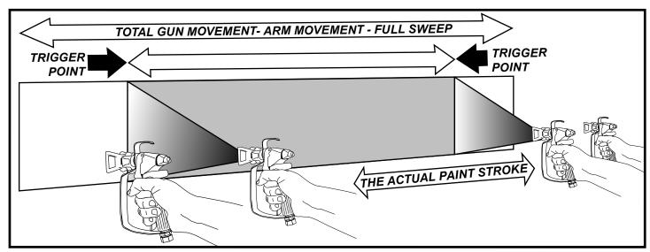
It is important to "trigger" the gun after gun movement (arm movement) has started and release trigger (shut gun off) before gun movement ends. Gun movement is always longer than actual paint (spray) stroke. In that manner, even blending and uniform paint coat thickness is achieved over the entire surface. When the gun is in motion as the trigger is pulled, it deposits an even amount of paint.
