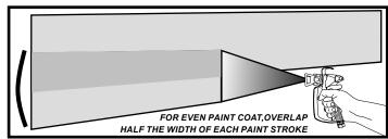
Spray with uniform strokes from left to right and from right to left, holding stroke speed, distance, lapping, and triggering as uniform as possible.
