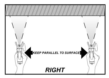
Move the gun at a steady rate in order to apply a good coverage. The wet coat should be just under the thickness at which a run or sag will occur. Slow gun movement or gun held too close will result in an overly wet or thick wet or thick coat coverage that is likely to run or sag.
