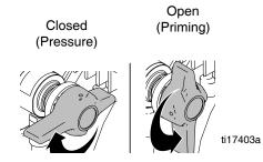
**NOTE:** The valve handle can move both clockwise and counter clockwise and can face different directions.
