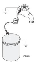
To maintain grounding continuity when flushing or relieving pressure: hold metal part of spray gun firmly to side of a grounded metal pail. Then trigger gun.
