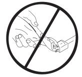
**Extension Cords:** Use an extension cord with an undamaged ground contact. If an extension cord is necessary, use a 3-wire, 12 AWG (2.5 mm<sup>2</sup>) minimum.
