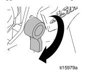
**Trigger Unlocked ASM 500**
