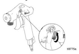
13. To achieve uniform spray pattern, adjust air valve and flow adjustment nut on gun. If you can not achieve a desired pattern, change nozzle, page 11.
