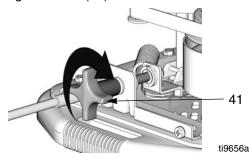
8. To set pressure, tighten knob (41) until back of bracket (25) is approximately 1/2 in. from front of tensioning bracket.
