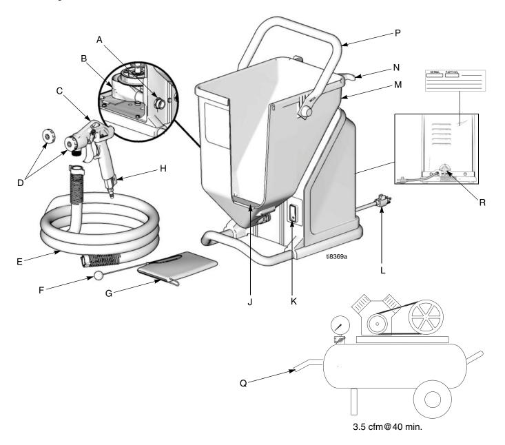
Item Component Item Component Pump Hose Outlet **Burp Guard** RotoFlex™ II Pump (inside) ON/OFF Switch K С Texture Spray Gun (Manual 311969) Power Cord (120V, 15 ft) Nozzle (2 included) Material Hopper - 5 gallon D М Ε Material Hose (20 ft) Ν Cord Wrap F Material Thickness Gauge Ρ Handle Air Compressor (Not Supplied) Accessories Bag G Q Н Gun Air Valve R Knob/Pressure Control
