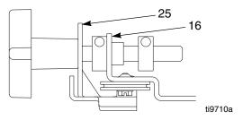
Tighten front spacer (56) until flush to front of tensioning bracket (16). Tighten back spacer (56) 3/8 in. from tensioning bracket.
