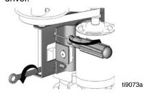
**NOTE:** Once the motor is in place, you can test the belt to make sure it is properly tightened. When you push on the belt (24) with one finger it should move no more than 1/4 in. If it moves more than 1/4 in., go back to step 8 and re-tighten the belt.
