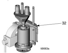
6. Use 9/16 in. wrench to loosen two mounting screws (4) on motor tray (32) to allow motor to slide around.
