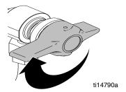
If the **spray tip or hose is clogged**, follow Steps 1 through 5 above. Expect paint to splash into the bucket while relieving pressure during Step 4.
