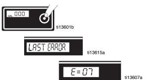
6. Press and hold DTS button to clear error code to zero.
