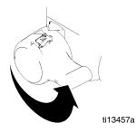
Hold gun against grounded metal flushing pail. Trigger gun and increase fluid pressure to 1/2. Flush 1 minute.
