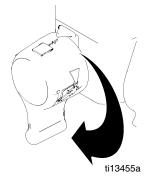
10. Place pump in grounded metal pail partially filled with flushing fluid. Attach a ground wire to pail and to true earth ground. Do 1. - 5. of **Startup** to flush out storage oil shipped in sprayer. Use water to flush water-base paint and mineral spirits to flush oil-base paint and storage oil.
