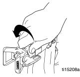
3. Turn pressure to lowest setting. Trigger gun to relieve pressure.
