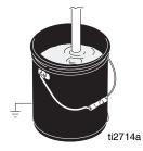
Trigger gun again into flushing pail until paint appears. Move gun to paint pail and trigger for 20 seconds. Set gun safety ON. Assemble tip and guard, see instructions on next page.
