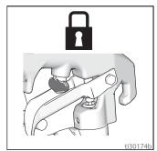
3. Remove tip and guard and disconnect gun from fluid hose.
