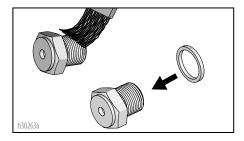
6. Screw diffuser/seat onto gun nozzle. Torque to 20-25 ft-lb (27-34 N•m).
