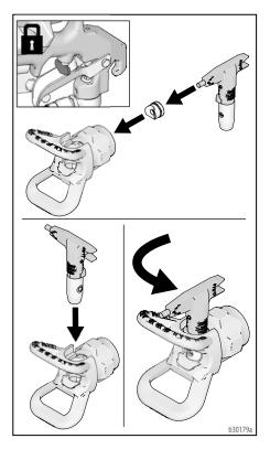
4. Screw spray tip and tip guard assembly on to the gun and tighten.
