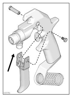
8. Attach tip and guard and attach gun to fluid hose.
