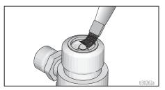
5. Grease threads of diffuser/seat. Place gasket on diffuser/seat.
