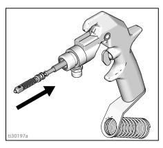
An insertion tool is provided in needle kit 235474. This tool helps prevent damage to needle.
