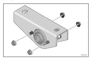
2. Slide each bracket-bearing assembly onto the axle, but do not tighten the bearing set screws.
