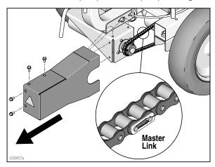
5. Disconnect the master link on the chain and remove the chain (316).
