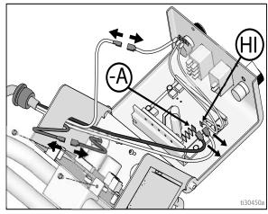
5. Remove the four screws to remove the switch housing, with the switch, from the mount.
