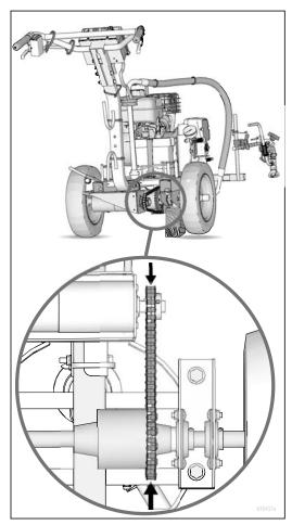
7. Turn OFF the self-propelled drive, place in "N", and replace the rear chain guard after sprocket alignment is confirmed.
