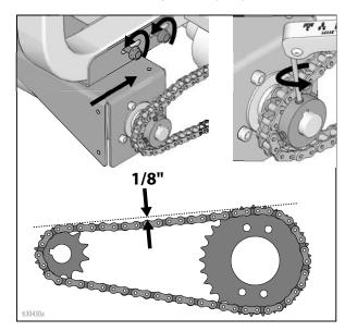
6. Remove the four screws (312) that secure the motor in the motor bracket (310) and slide the sprocket off of the motor shaft while removing the motor (311).
