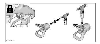
3. Screw assembly onto gun. Hand tighten.
