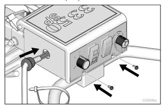
5. With the self-propelled drive system switch in the OFF position, and the drive switch in "N", connect the battery or insert the fuse.
