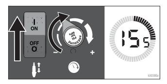
10. Turn pressure down, close prime valve. Disengage gun trigger lock.
