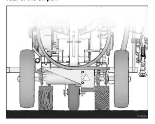
3. While holding the wheel (3) to keep the axle from spinning, loosen and remove the axle nut (307). Slide the wheel off the axle (300) making sure to retain the key (306).
