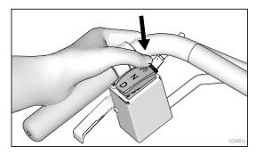
With a clear and safe path ahead of the striper, and with one hand on the left handlebar, slowly turn the speed knob clockwise until the desired speed is achieved on the specific terrain.
