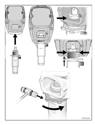
4. Fill packing nut with TSO until fluid flows onto the top of seal. Install pump rod cover (107).
