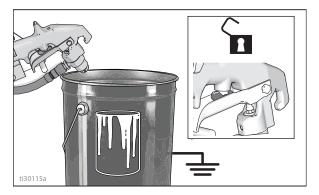
Gradually turn pressure control up until motor begins to drive pump. Trigger gun until flushing fluid appears.
