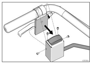
6. Unplug the wire harness from the switch and remove the drive switch from the housing.
