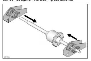
3. Bolt the axle assembly to the frame and torque to 30-40 ft-lb  $(40.7-54.2 \text{ N}\cdot\text{m})$ .
