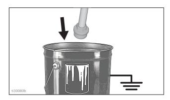
14. Trigger gun again into flushing fluid pail until paint appears. Assemble Uni-Tip and Uni-Tip Guard.
