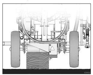
3. While holding the wheel (3) to keep the axle (300) from spinning, loosen and remove the axle nut (307). Slide the wheel off the axle making sure to retain the key (306).
