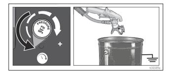
4. Engage the trigger lock. Turn prime valve down.
