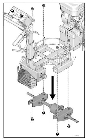
7. Loosen all of the bearing (303) set screws and slide each bracket-bearing assembly off of the axle (300).
