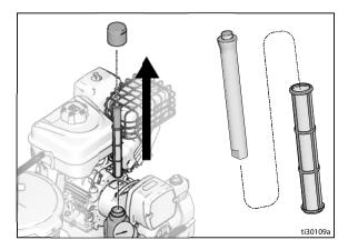
4. Clean gun filter, Uni-Tip Guard and Uni-Tip in flushing fluid. See **Flushing Recommendations**, page 23.
