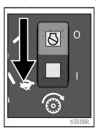
3. Move the Engine Kill/Drive Power switch to the middle position to shut off the drive system. Fully depress the top portion of the Engine Kill/Drive Power switch to shut off the gas engine. The drive system is off when the green light on the switch is off.
