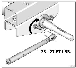
5. Align the axle sprocket with the motor sprocket, place a drop of blue thread locking liquid on each bearing set screw and tighten all set screws.
