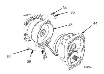
4. Place pinion assembly (44) on bench with rotor side up.
