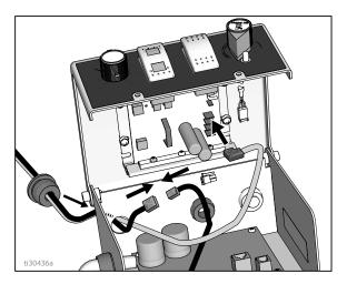
6. Reconnect the battery (321) or replace the fuse. Turn ON the self-propelled drive. With the brake ON and the right wheel securely elevated just enough to be off of the ground, run the drive. If any noise or binding occurs at the chain, realign the motor sprocket (313), or adjust the chain slack.
