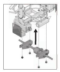
4. If bearings were replaced, torque the nuts (305) and bolts (304) to 23-27 ft-lb (31.2-36.6 N·m).
