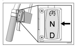
2. Press the bottom portion of the Engine Kill/Drive Power switch to power the drive system.
