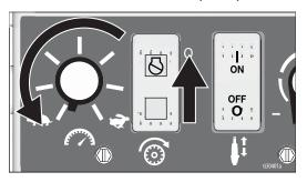
2. Press Cruise (3) on the driver control switch to engage the self-propelled drive.
