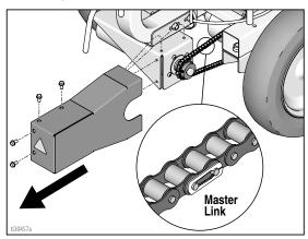
3. Disconnect the master link on the chain and remove the chain (316).
