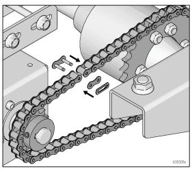
2. If the chain cannot be connected, or the chain slack needs adjusting, loosen the two motor bracket bolts (314) and slide the motor forward or backward as needed. Re-torque to 30-40 ft-lb (41-54 N·m).
