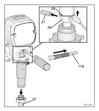
5. Loosen jam nut by hitting firmly with a hammer. Unscrew pump.
