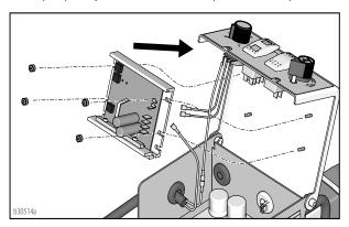
2. Connect the eight wires as shown (as indicated per the wire labels).
