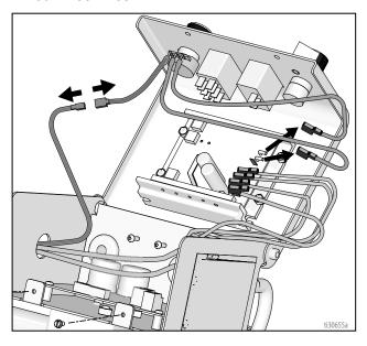
3. Remove the speed knob (62h) using a 5/64" allen wrench, the friction o-ring (62k), the retaining nut, and the spacer (62g).
