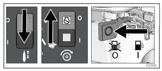
Turn pressure to lowest setting. Trigger gun to relieve pressure.
