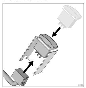
2. Install the four screws to attach the switch and switch housing to the mount.
