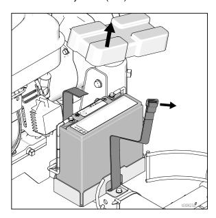
3. Unscrew M5 terminal screws (358) to disconnect battery from wire harness.
