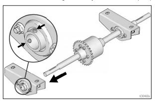
8. If replacing the axle bearings, unbolt each bearing (304 and 305) from the axle bracket (302).
