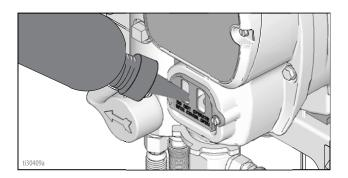
3. Check engine oil level. See Briggs & Stratton engine manual.
