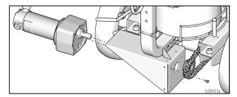
3. Slide the motor bracket (310) back to leave about 1/8" slack in the chain (316), and tighten the motor mount bolts (314). Torque to 30-40 ft-lb (41-54 N·m).
