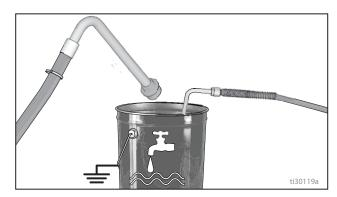
13. Set pump switch **OFF.** Turn engine **OFF** by pressing the engine kill switch at the controls, or by moving the lever on the engine.
