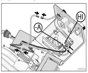
4. Replace the strain relief bushing (333) and close control box cover (62a).
