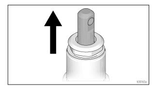
2. Push pin (31) into hole. Push retaining ring spring into groove all the way around connecting rod.
