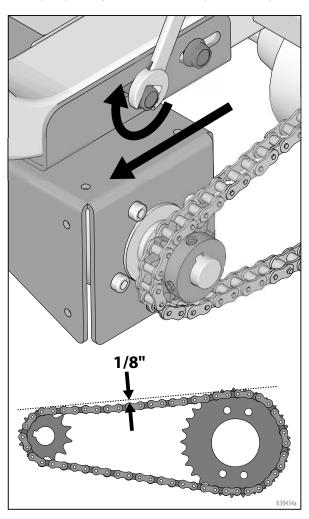
4. Adjust the motor sprocket (313) so that it is in-line with the axle sprocket, then place a drop of blue thread locking liquid onto the threads of each set screw and secure the motor sprocket in place. Torque to 50-60 in-lb (5.6-6.8 N·m).
