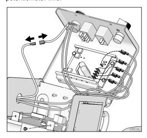
4. Unscrew the 4 mounting nuts (62f) and remove the control board (62e) from the control box cover (62a).
