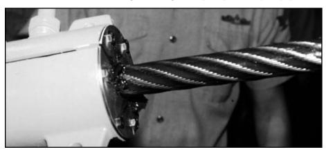
viscous lubricant is applied to the surface of the wire, only served to trap any corrosion inside causing moisture, while the spraying method which utilized thin lubricants through a spray nozzle applicator, provided minimal fluid film barrier between individual wire strands allowing excessive friction wear.
