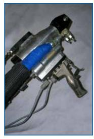
The new gun eliminated the need for a hot water purge required on the dynamic mixer setup, which increased productivity and reduced the waste stream.
