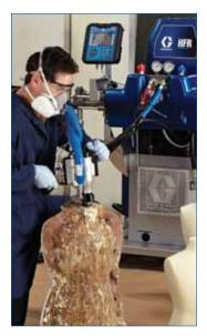
The system's Advanced Display Module (ADM) allowed Ronis to program multiple pour shots for multiple size molds. This eliminated downtime between line changeovers, increasing overall productivity and uptime. Having the ADM available in Spanish was a substantial added benefit for this facility.
