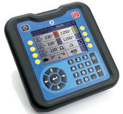
Figure 8 – The Advanced Display Module provides an easy to use interface with detailed error codes, troubleshooting help, and data logging
