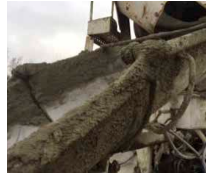
Dried concrete on a discharge chute was a major problem for concrete mixing plant.
