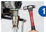
Loosen the clamping nut
