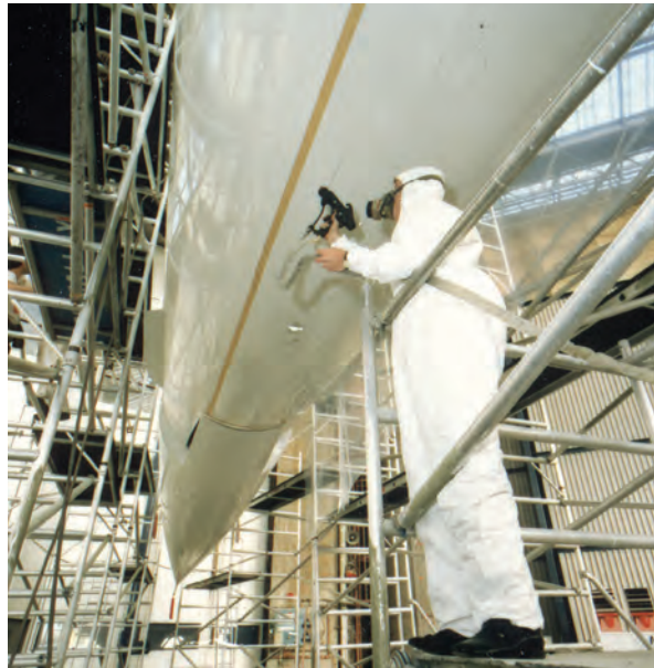
PRO AA4000 electrostatic air-assisted airless spray gun used to paint the Concorde supersonic jet aircraft.
