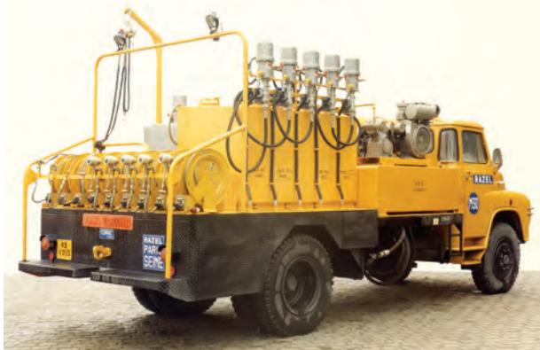
Mobile Lube Ranger® designed and built by Fog used to supply road contractors with on-site lube service for heavy equipment.
