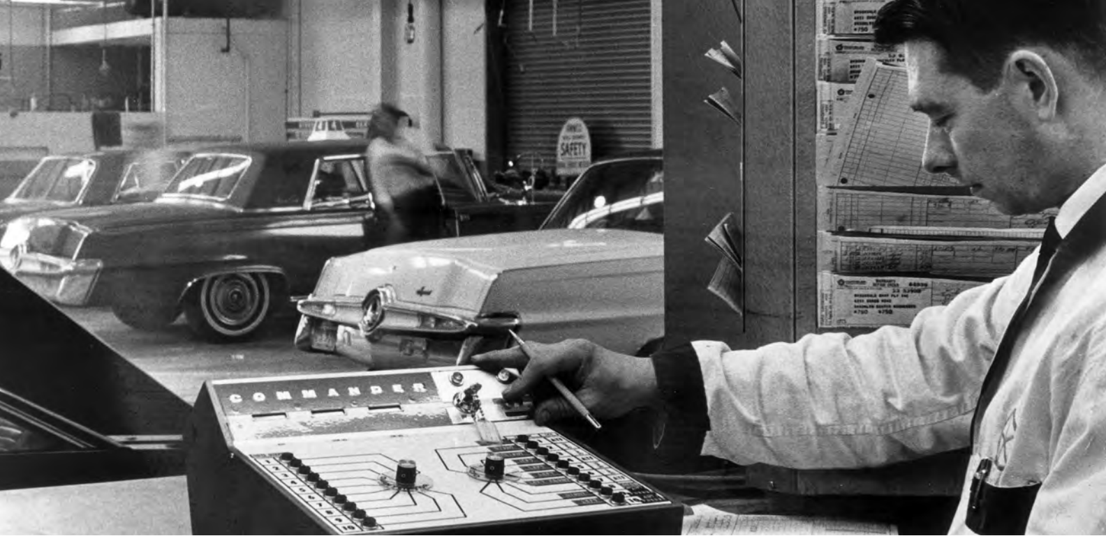
Fluid Commander™ is an automated system for controlling, metering and keeping inventory of dispensed automotive fluids.
