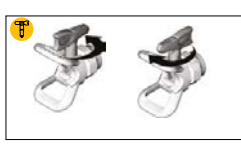
To clean clogged tip, turn applicator OFF, turn tip 180° to CLEAN position, aim towards free area, turn applicator ON. When clog clears, turn applicator OFF and tip to SPRAY position.
