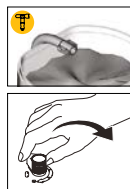
Turn pressure control knob until steady stream flows from product tube.
