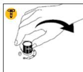
Turn pressure control to maximum. To spray, aim applicator at wall from 0.5 m distance wall and open applicator.
