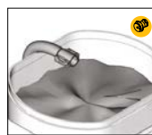
Place product tube into hopper, turn ON/OFF switch to ON. Turn control knob to 'green' section and allow material to product 30 sec.
