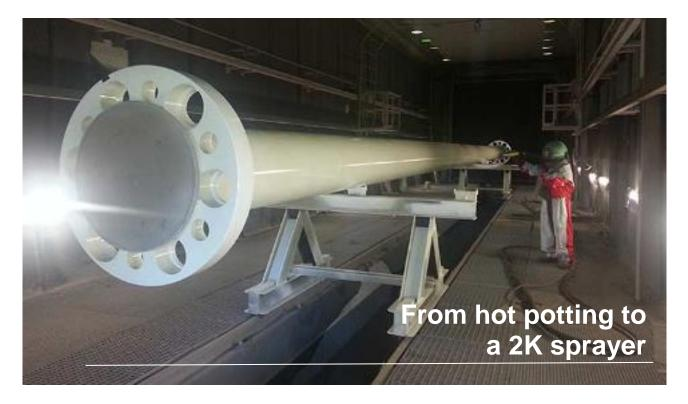
Freeman France, a subcontractor of Cameron, is based in South of France at Beziers. They specialize in coating large or oversized pipes used in petroleum pumping plants. The automatic painting applications are done in Cameron's facility. Freeman paints pipes in very different sizes. This is done via a manual application, hot potting high performance paint.
