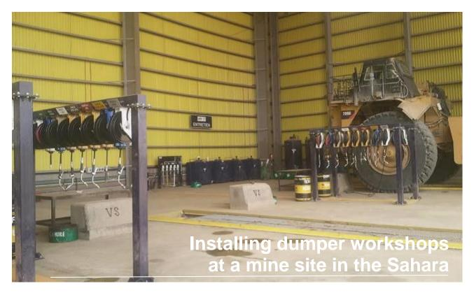
A large mining company in Mauritania needed to improve their facility to handle the increasing maintenance of dumpers. They were dealing with problems such as pollution, sand, high outside temperatures (40 to 50°C), and dust due to poor working conditions and the use of inappropriate equipment. Fuel dispensers were used to manually transfer lubricants and grease which meant there was a lot of wastage and mishandling of lubricants, resulting in time-consuming maintenance for the employees.
