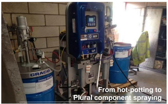
Founded in 1975, Snashall Steel Fabrication is a British manufacturer of steel frame structures for a variety of businesses. Their existing paint process was based upon hot-potting of materials via a low pressure single leg pump. With an increasing production and a growing business, Snashall identified the need to move from hot-potting to plural component spraying.
