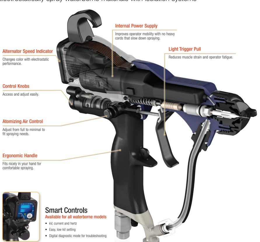
High transfer efficiency for low or high pressure applications
