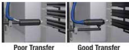
Dual shaping air can also help reduce unnecessary space on your paint line, especially when it's time to change colors or clean equipment.
