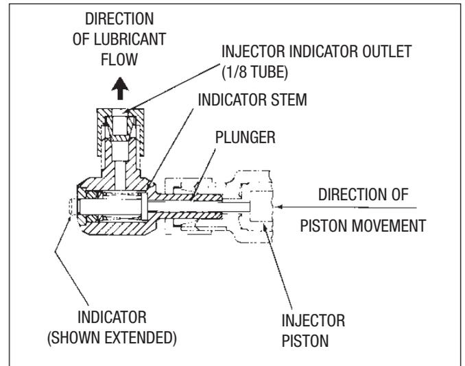
**Figure 13. Injector Cycle Indicator
