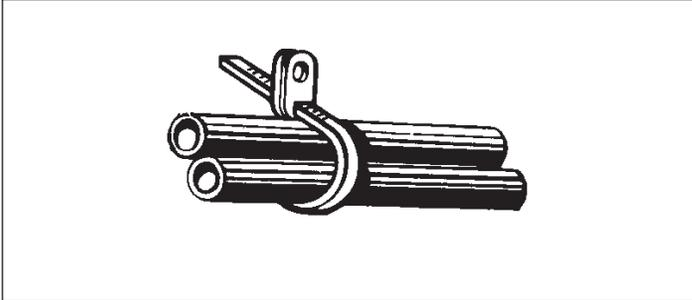
Figure 20. Tubing Straps
