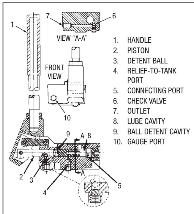
**Figure 6. Hand-Operated Pump - Operation
