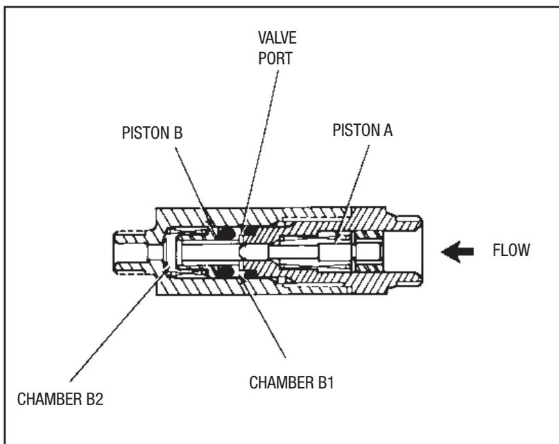
Figure 12. Injector Operation
